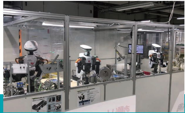
Kasugai Plant Collaborative robot assembly line
