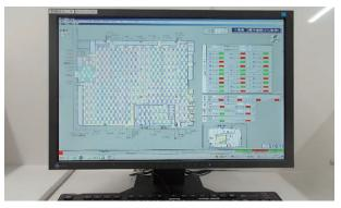
At our Tohoku Plant, we have installed a Factory Energy Management System (FEMS) which can visualize energy management from power receiving to distributing to facilities, monitoring energy use, operational status of production and infrastructure equipment, and energy consumption. By measuring and analyzing the energy consumed by each equipment, we can optimize plant energy usage and reduce CO<sub>2</sub> emissions.
